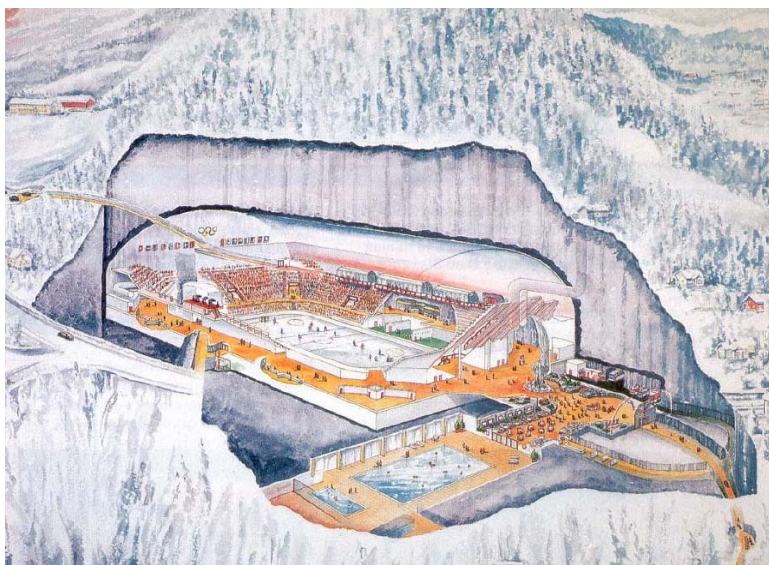
Underground stadium 90 x 60 x 25 m
